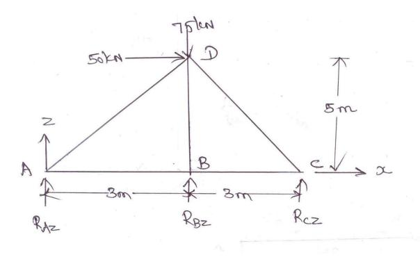
2. Analyse the space truss shown in the figure by the method of tension coefficients and determine the member forces.
