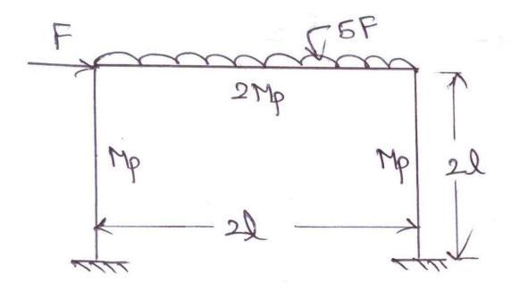
10 Find the collapse load for the loaded frame loaded as shown.
