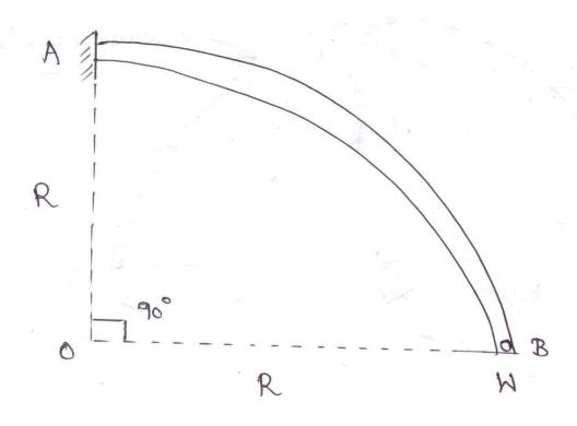
3. A curved beam AB of uniform cross section is horizontal in plan and in the form of a quadrant of a circle of radius R. The beam is fixed at A and free at B.It carries auniformly distributed load of w/unit run over the entire length of the beam as shown. Calculate the shear forces, bending moment and Twisting moment value, at A and B and sketch the variations of the same. Also determine the deflection at the free end B.
