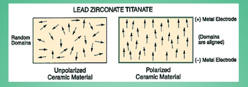
FIG: a) RANDOM ORIENTATION OF DOMAINS PRIOR TO POLING.b) REMANENT POLARIZATION AFTER FIELD IS REMOVED.
