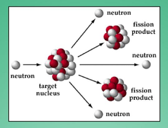
The reactor uses Uranium rods as fuel, and the heat is generated by nuclear fission.
