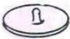
Fig 1.17: Adhesive tape electrode [Source: Leslie Cromwell - Biomedical instrumentation and measurement]
