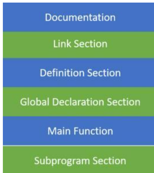
Fig1: Basic Structure of a C Program
