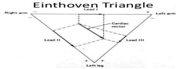
The vector sum of the frontal plane Cardiac Vector at any instant onto the three axes of the Einthoven Triangle will be zero.
