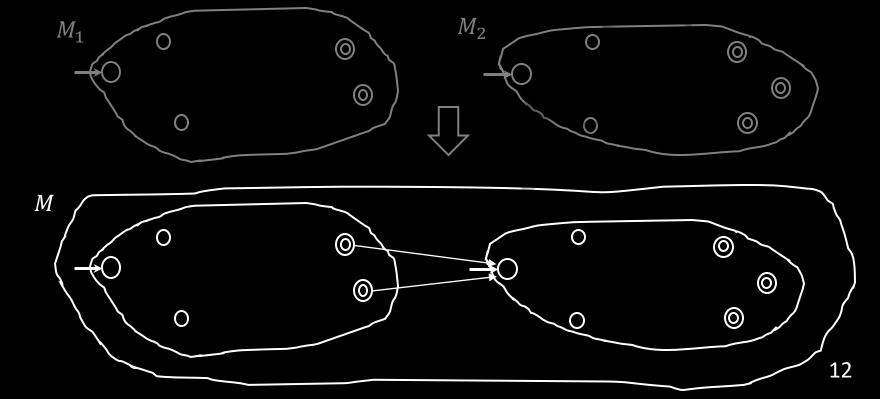
M should accept input w if w = xy where  $M_1$  accepts x and  $M_2$  accepts y.
