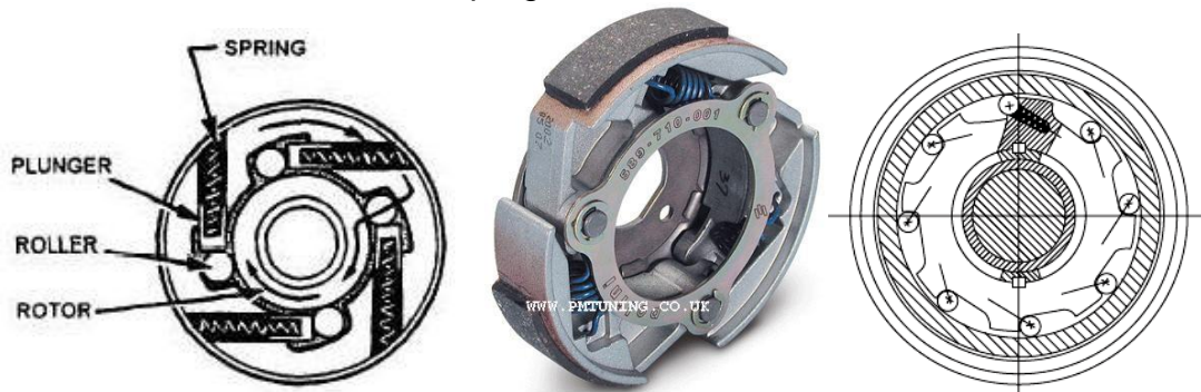
Roller-type freewheel, with rollers retracted against their springs
