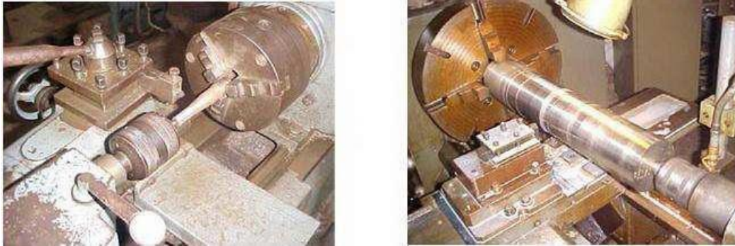
Fig. 2.19 Work held between chuck and revolving centre
