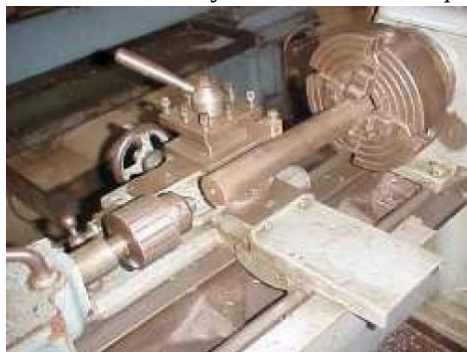
Fig. 2.24 Holding drill chuck and drill in tailstock
