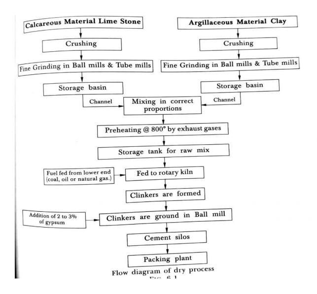
The most common way to manufacture portland cement is through a dry method. The first step is to quarry the principal raw materials, mainly limestone, clay, and other materials. After quarrying the rock is crushed. This involves several stages. The first crushing reduces the rock to a maximum size of about 6 inches. The rock then goes to secondary crushers or hammer mills for reduction to about 3 inches or smaller.
